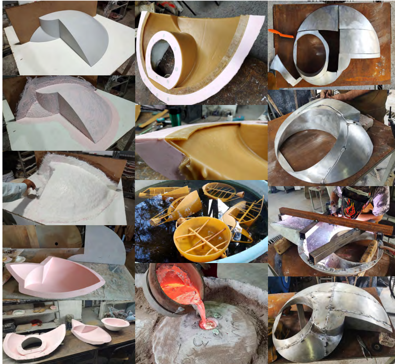
From 3D print to aluminum cast at Art21Studio in Zapopan, Jal., Mexico
